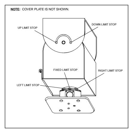
Figure 4. PT573R/PT573-24R Limit Stop Adjustments
